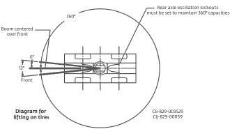
Bold lines determine the limiting position of any load for operation within working areas indicated.
